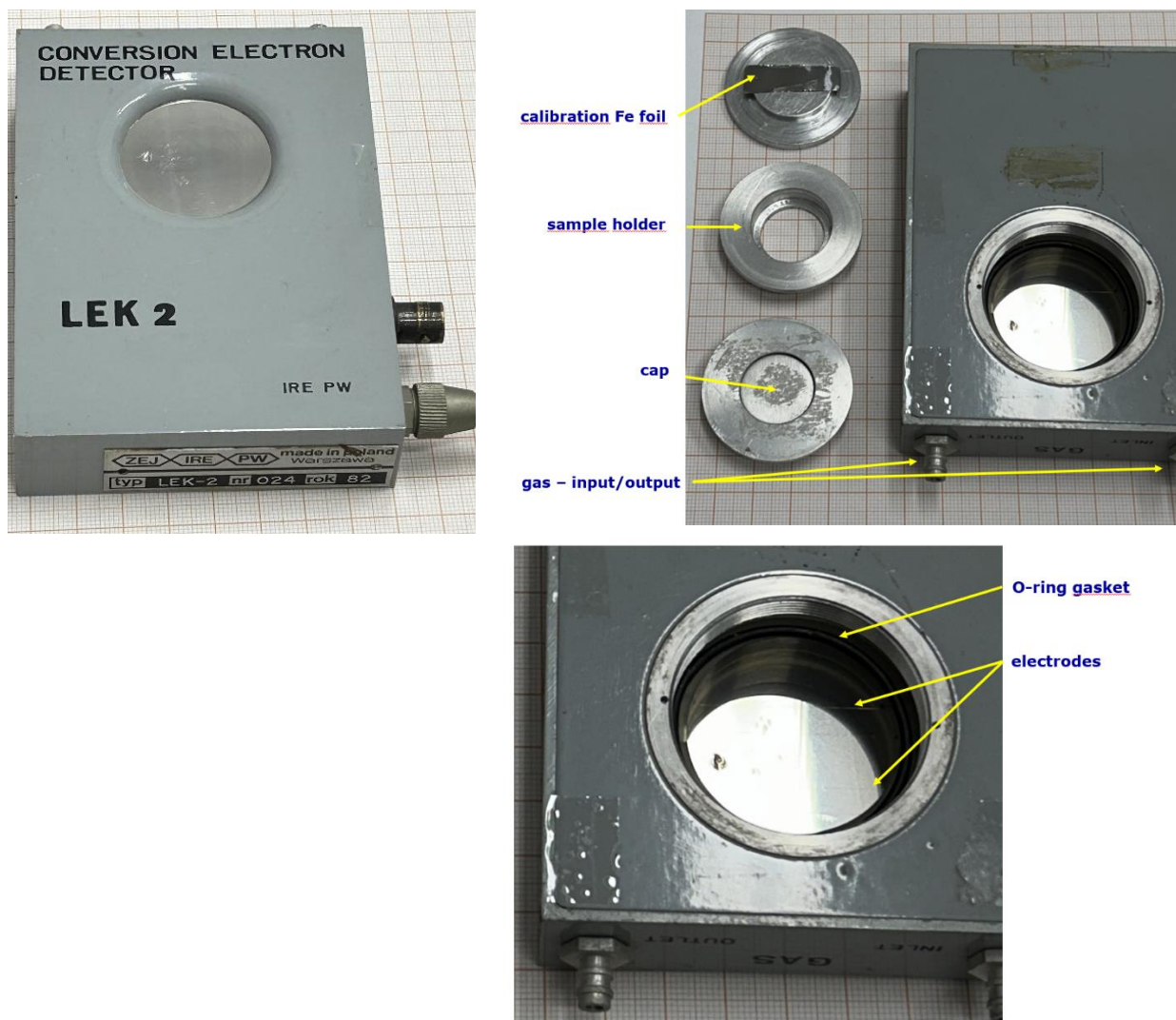
Figure 6. The LEK 2 conversion electron detector.
